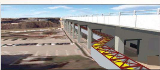
Actual Model created using Survey and Mapping Datasets, Regional GIS Datasets, AutoCAD Civil 3D Design and then consolidated using Autodesk Infrastructure Modeller.
